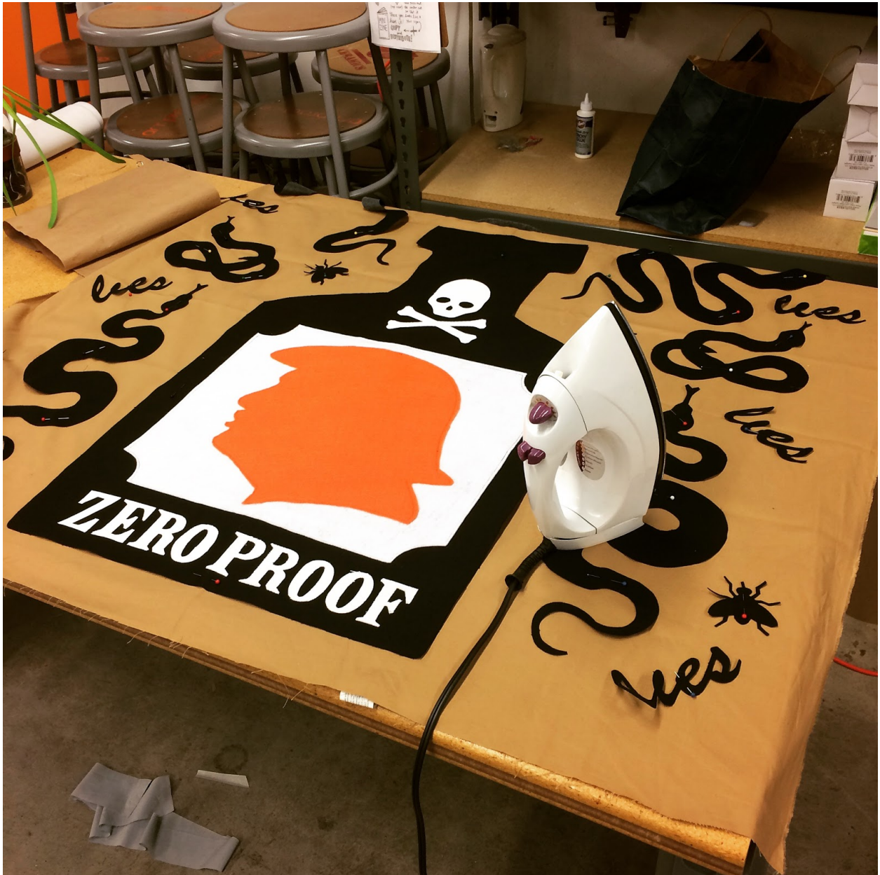
Laying out the pieces on a large table and pinning together. An ironing pad is underneath and the components are first ironed down and then topstitched.
